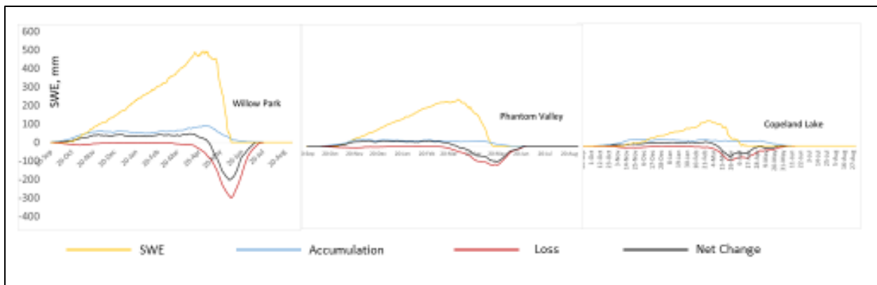
Figure 4.12. Fifteen-day changes in SWE, along with the average niveographs, for three SNOTEL stations.
