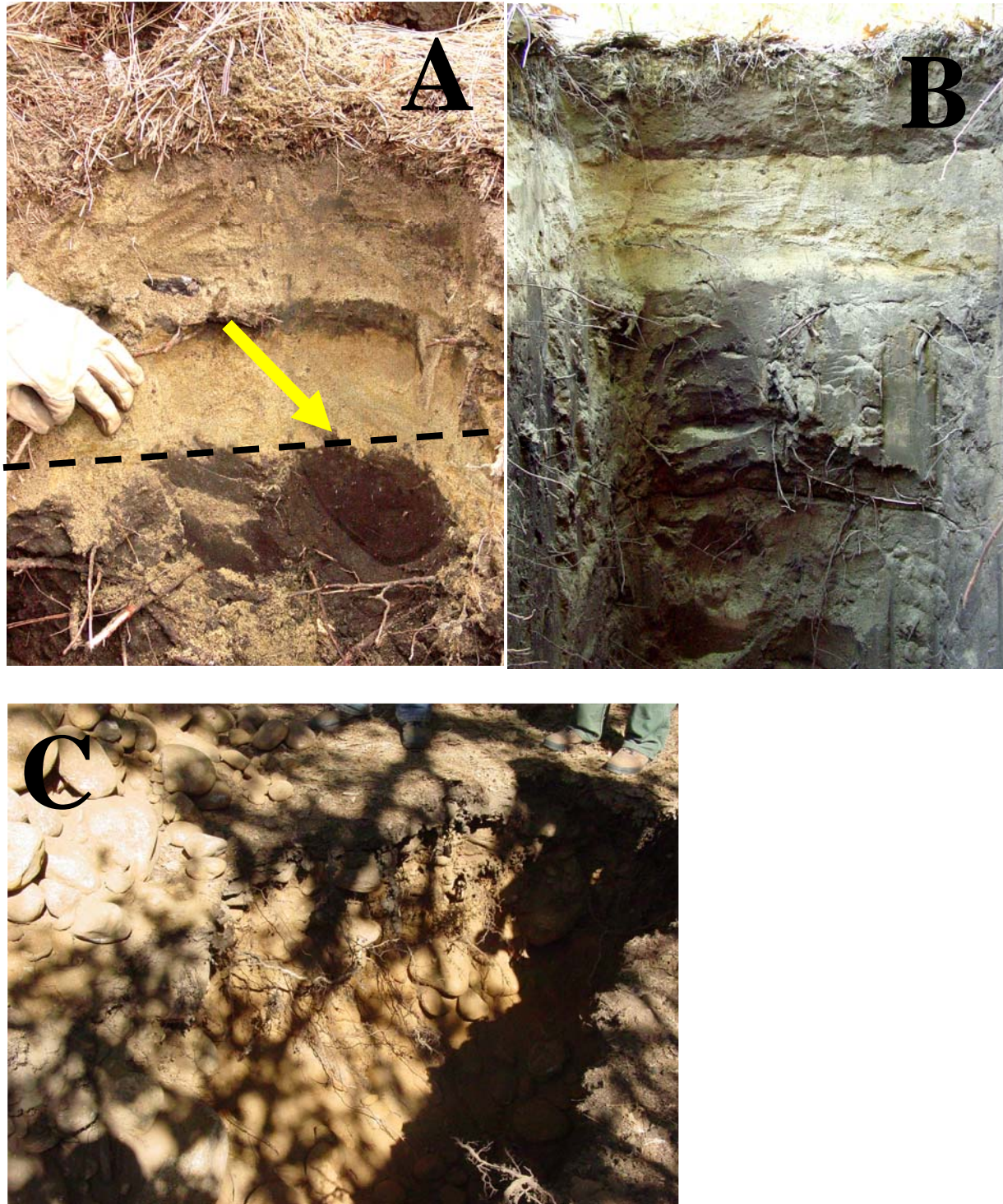
Figure 26. Three soil profiles in backhoe pits. A shows a very dark, organic rich soil (below dashed line) with some sandy layers above. B shows a dark surface horizon, a sandy buried soil, and a dark buried soil below the sand. C shows a cobble soil.
