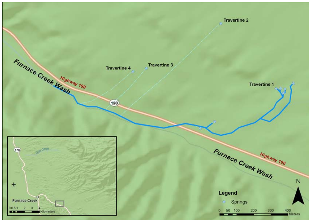
Figure 2. Schematic drawing of the Travertine Springs Province. Blue lines represent existing springbrooks, and light blue, dashed lines represent possible springbrook routes that will exist when discharge from Travertine Springs 2, 3, and 4 are released onto the land surface.
