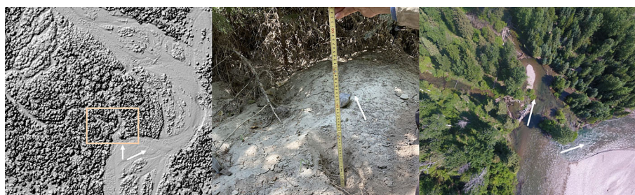
FIGURE 6 An avulsion on the Swan River downstream of Goat Creek (Figure 3 for location within catchment). The first return hillshade from lidar is on the left, ground view of floodplain vertical accretion during 2022 peak flows is at the centre, and the drone photograph is on the right. The pink box denotes the location of the avulsion. Arrows indicate flow direction. [Color figure can be viewed at wileyonlinelibrary.com ]
