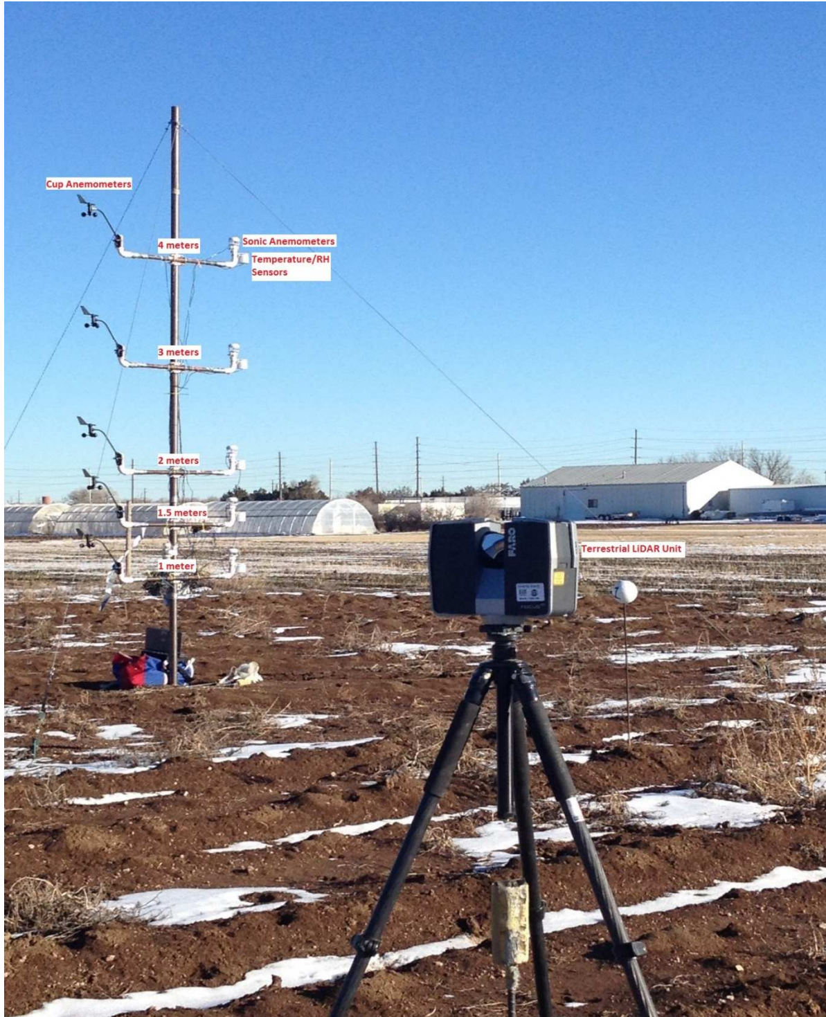
Figure 1: Terrestrial LiDAR scanner and instrumented meteorological tower at the study site.
