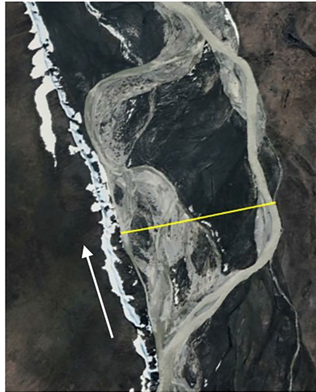
Figure 2. Example of measuring channel migration zone width, here on the Echooka River at 69.41683, -148.08508 . The yellow line is 520 m long. White arrow indicates flow direction.
